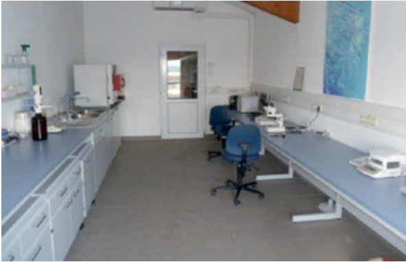
Figure 15 Small-scale laboratory at an Austrian biogas plant. Minimum laboratory equipment consists of a pH-meter, a drying oven and a muffle furnace. Additional instrumentation for determination of \text{NH}_4\text{-N} and titration systems (alkalinity ratio or total VFA) are recommended (reproduced with the kind permission of R(o)HKRAFT).
