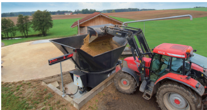
Figure 3 The solid feedstock is loaded into an automatic feeding system which records the mass input fed into the biogas plant (reproduced with the kind permission of Fliegl Agrartechnik).
