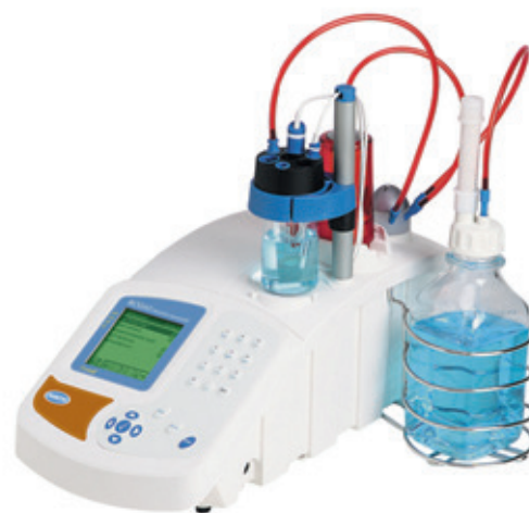
Figure 12 Automated laboratory titration device (reproduced with the kind permission of HACH LANGE).
