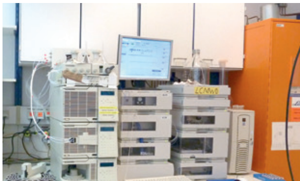
Figure 11 High pressure liquid chromatography (HPLC) measuring system for the determination of individual VFA
